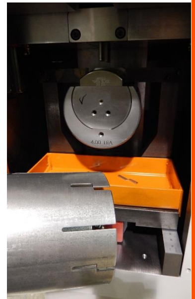
SLOT-200 MACHINE: Cuts one slot at a time is powered by shop air instead of hydraulics. This is our budget model
